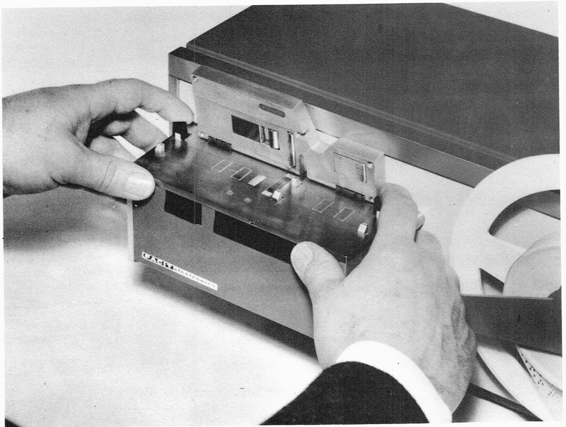
Fig. 5 - 5 Changeover to different tape width
