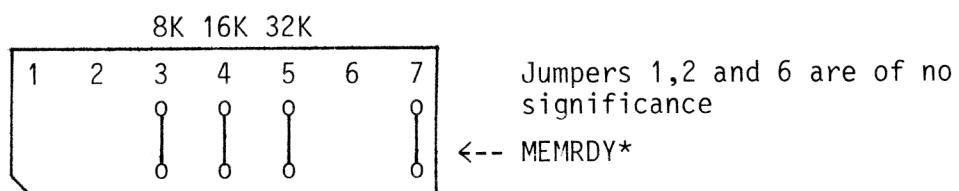
The MEMRDY\* jumper installed = wait-state signalling connected.
