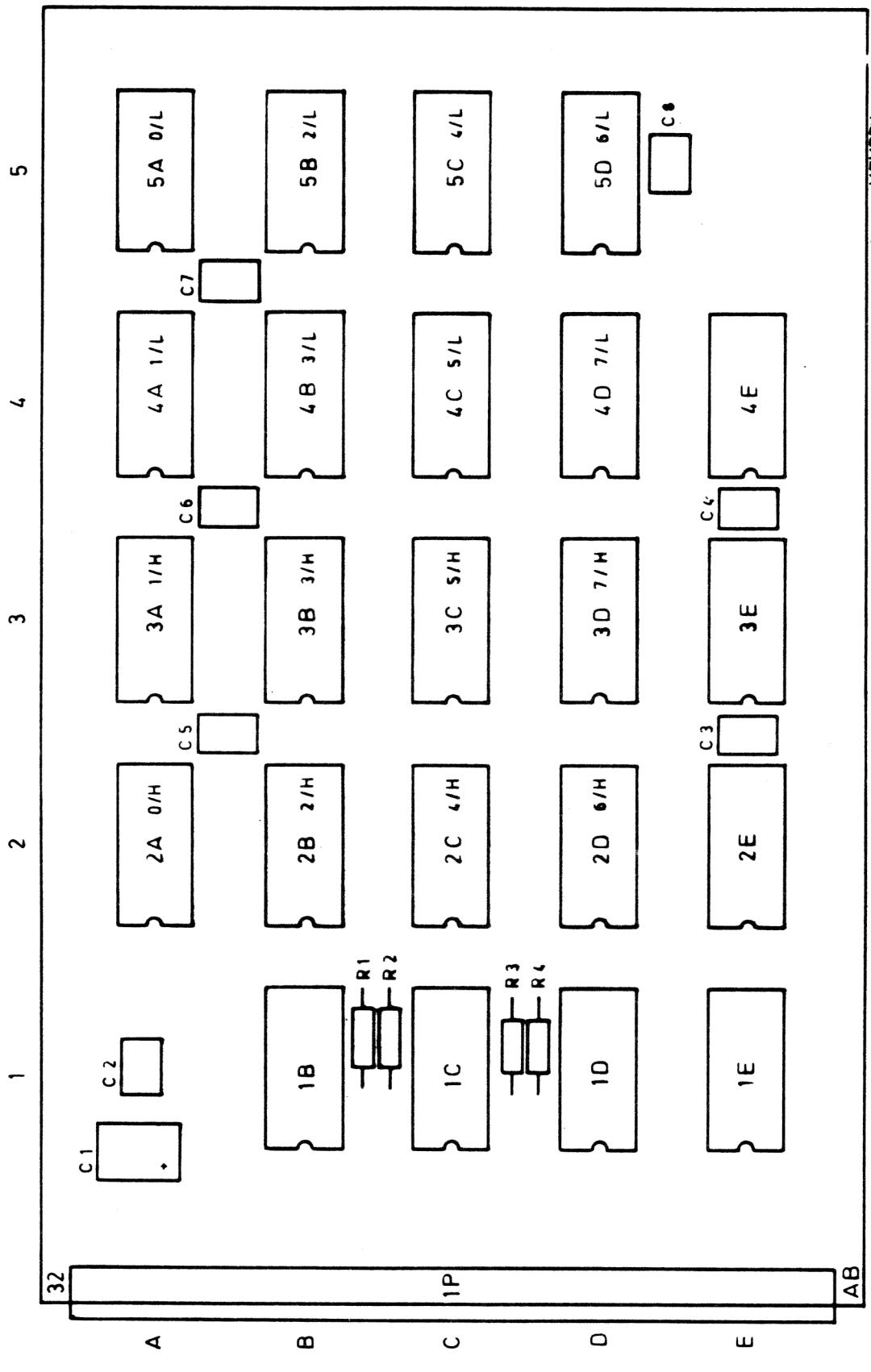
NOTE MEMORY ADDRESS IS SPECIFIED FOR EACH MEMORY CIRCUIT. THE FIRST 1k ARRAY IS PLACED IN '2A' FOR HIGH ORDER BITS (7-4) AND 3A FOR LOW ORDER BITS (3-0).
