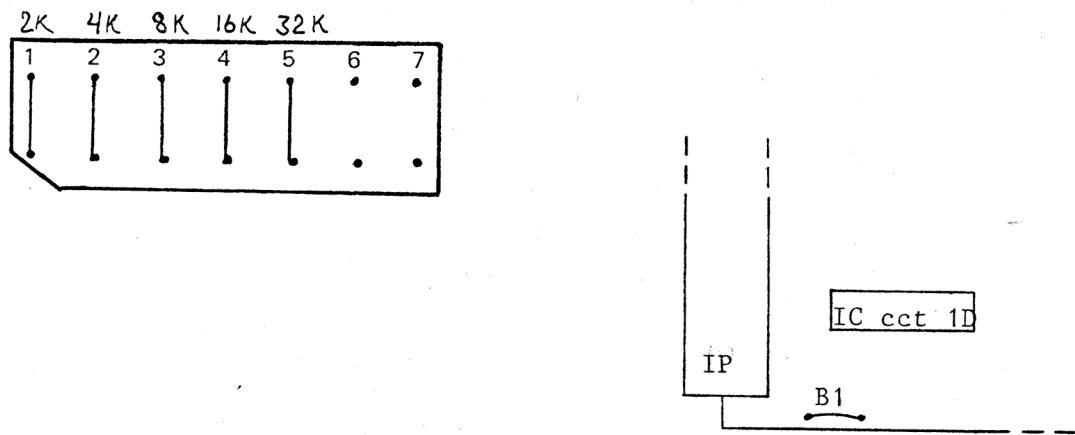
The MEMRDY\* -signal is connected to the bus-connector by jumper B1 located directly beneath the IC-circuit 1D.
