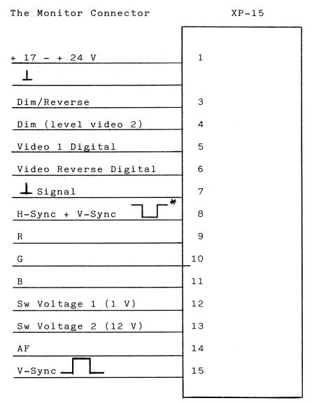
\*Sync: If H-sync and V-sync signals are separated, they should be connected to the following pins: o H-sync - pin 8. o V-sync - pin 15.
