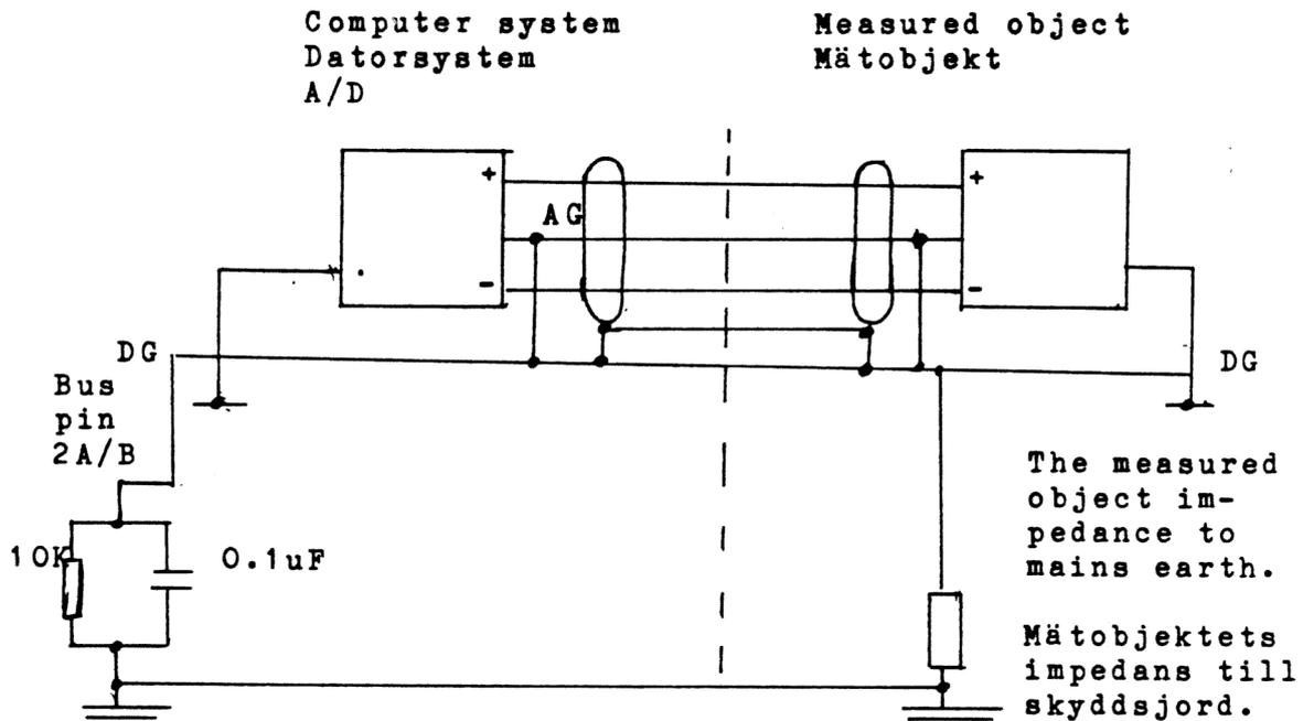
The 10K/0.1uF protects against disturbance from static electricity, connected between mains earth and digital ground.
