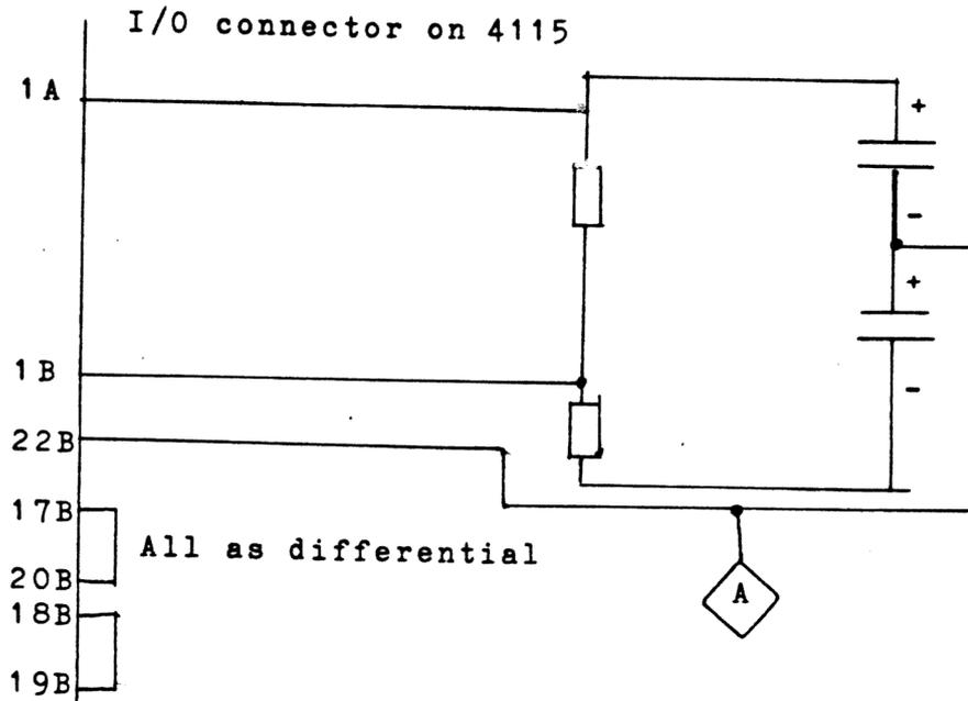
Note! A is system ground, which must be connected to the analogue ground at the signal source.
