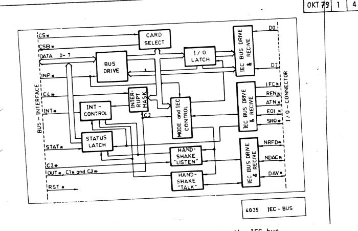
4025 provides DATABOARD 4680 users interfacing to the IEC-bus.
